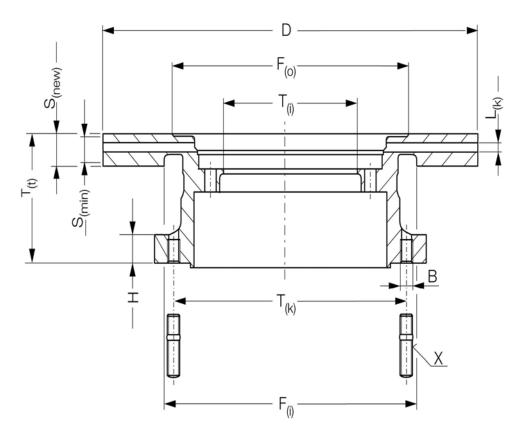
B Diameter of mounting bolt holes (or thread size in case of threaded holes)
