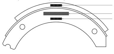
Make and type of brake lining Date of assembly manufacture and manufacturer's name or trade mark Approval mark
